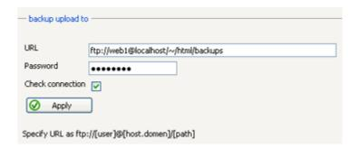
Specify a link for backup upload in the "URL" field. The link must be in the following format: <a href="ftp://(user)@(host.domain)/(path)">ftp://(user)@(host.domain)/(path)</a>. Enter your password for the external FTP resource you're uploading to and click "Apply" to confirm. If you wish to check data validity during connection with the FTP server, tick the "Check connection" box.
